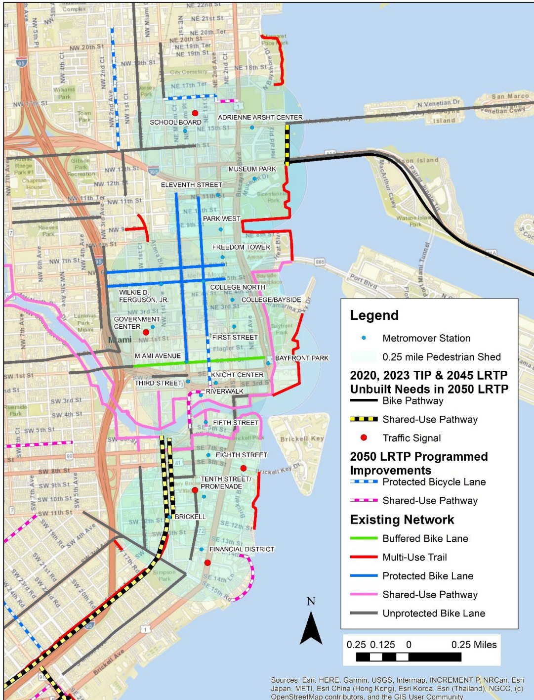
Map 6. Metromover stations pedestrian shed analysis of existing and proposed bicycle network improvements in the study area.
