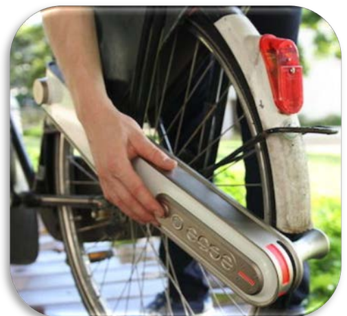
Figure 103. Portable propulsion devices can convert conventional bikes to e-bikes.
